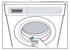
3. Leave the appliance door and detergent drawer open so that residual water can evaporate.
