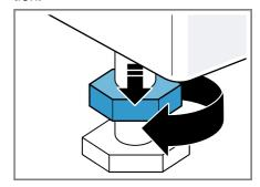
To align the appliance, turn the appliance feet. Check that the appliance is level using a spirit level.
