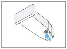
Check the condensation container filter → Page 40 regularly and clean the filter if it is dirty. Make sure that you insert the condensation container before operating the appliance.
