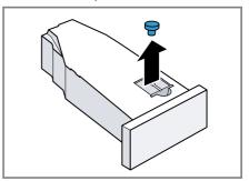
2. Insert the stopper on the underside.
