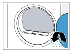
3. Remove the two-part fluff filter.
