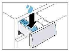
**5.** Add washing powder containing oxygen bleach to the manual dosing compartment.
