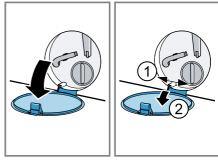
Slide a suitable receptacle under the opening for draining the detergent solution.
