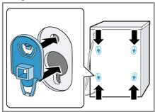
If one cover cap is included in the scope of delivery, insert the cover cap in the bottom left opening for the transit bolt.
