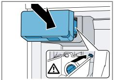
If, during fitting, the ice storage container is blocked, remove the excess ice cubes from the ice storage container opening.
