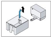
3. Insert the suction hose with connecting piece into the opening of the pump cover, turned 180°.
