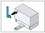
**4.** Carefully put approx. 15 ml drinking water into the suction hose with connecting piece.
