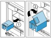
**2.** Remove the suction hose with connecting piece from the water tank.
