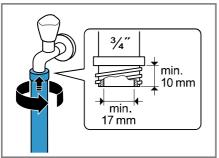
**3.** Open the water tap carefully and check that the connection points are tight.
