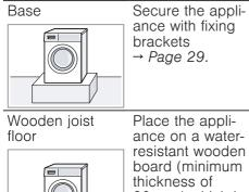
resistant wooden board (minimum 30 mm) which is screwed tightly to the floor.
