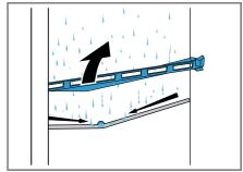
2. Carefully clean the condensation channel and the drainage hole, e.g. using a cotton bud.
