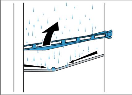
2. Carefully clean the condensation channel and the drainage hole, e.g. using a cotton bud.
