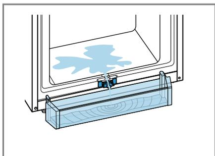
6. To collect the condensation, remove the shelf for large bottles from the refrigerator door and place it below the open condensation outlet.
