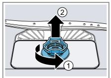
Pull down the micro filter to remove.
