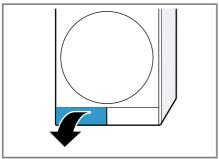
If you place a cloth beneath the maintenance flap, you can collect the remaining water from the base unit.
