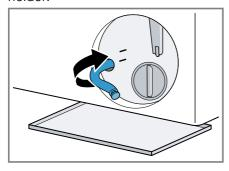
**Cleaning the drain pump Requirement:** The drain pump is empty. → *Page 31*
