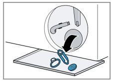
**3.** Ensure that both impellers can turn.
