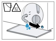
8. Firmly press on the sealing cap.
