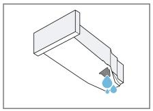
Check the condensation container filter → Page 37 regularly and clean the filter if it is dirty. Make sure that you insert the condensation container before operating the appliance.
