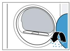
3. Remove the two-part fluff filter.
