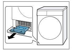
**4.** Clean the insert under running water and dry it off.
