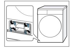
3. Pull out the heat exchanger cover by the handle.
