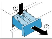
3. Pull out the insert upwards.
