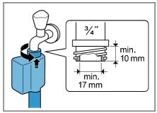
2 Open the water tap carefully and check that the connection points are tight.
