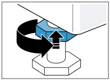
In doing so, hold the foot tight and do not adjust its height.
