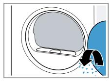
3. Remove the two-part fluff filter.
