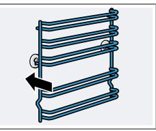
The rails fit both on the left and right sides. Shelf positions 1 and 2 are located at the bottom and shelf positions 3, 4 and 5 are located at the top.
