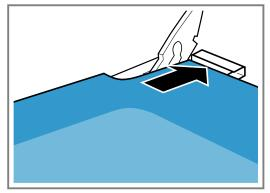
Push the pane into both openings on the underside. The smooth surface of the pane must face outwards.
