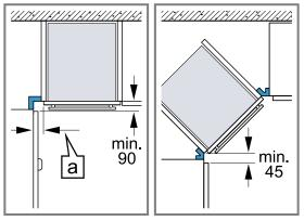
Observe the minimum dimensions in a corner installation in order to be able to open the cover of the appliance. The dimension a depends on the thickness of the furniture panel and the handle.
