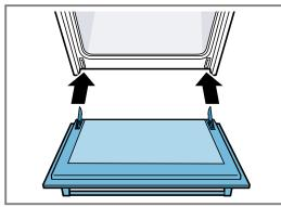
2. The notch on the hinge must engage on both sides.
