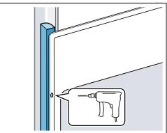
4. Secure the appliance using a suitable screw.
