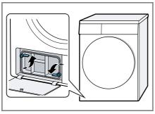
**3.** Pull out the heat exchanger cover by the handle.
