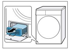
4. Clean the heat exchanger from all sides under running water and dry it.
