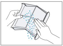
Clean the fluff filter thoroughly under warm, running water and then dry it off.
