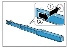
2. Place the telescopic rail on the rear pin ① and push the locking mechanism back 2.
