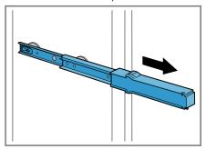
2. Move the lock in the direction of the arrow ① and loosen the pin from the rear ②.
