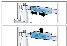
You can remove the door rack rail and re-insert it elsewhere.
