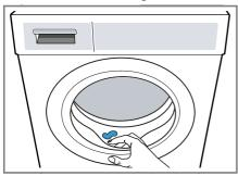
Clean the outside and the inside of the rubber gasket with a damp cloth and wipe dry.
