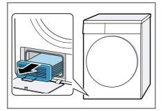
4. Clean the heat exchanger from all sides under running water and dry it.
