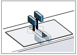
6. Insert the grease filter.
