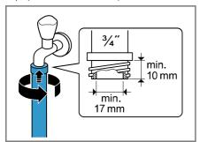
3. When connecting to a 21 mm = ½" tap, first fit the adapter with a sealing washer.
