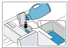
Do not exceed the marking for the maximum filling level when filling.
