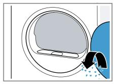
3. Remove the two-part fluff filter.
