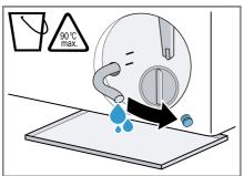
8. Firmly press on the sealing cap.
