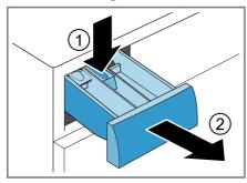
3. Pull out the insert upwards.
