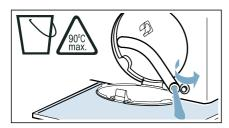
4. Carefully unscrew the pump cover; residual water may leak out. Clean the interior, pump cover thread and pump housing. The impeller in the drain pump must be able to rotate.
