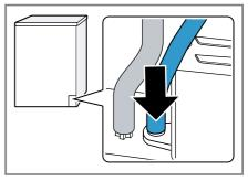
**4.** Insert the water outlet hose into the hose guide.
