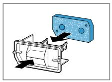
Ensure that the cleaned filter mat is not deformed, damaged or inverted when you push it onto the retainers.
