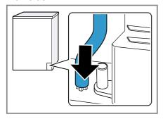
**3.** Push the water outlet hose as far as it will go into the connecting piece.
