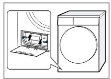
**3.** Pull out the heat exchanger cover by the handle.
