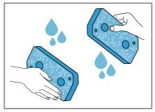
You can remove heavy soiling carefully using a vacuum cleaner. Do not clean the filter mat using cleaning agents.
