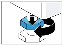
2. To align the appliance, turn the appliance feet. Check that the appliance is level using a spirit level.
