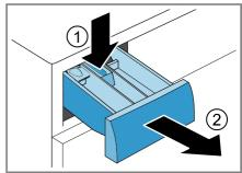
**3.** Pull out the insert upwards.
