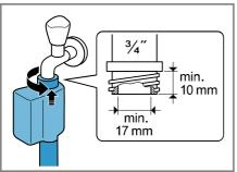
2. Open the water tap carefully and check that the connection points are tight.
