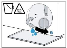
8. Firmly press on the sealing cap.
