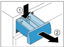
3. Pull out the insert upwards.
