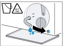
8. Firmly press on the sealing cap.
