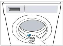
4. Leave the appliance door and detergent drawer open so that residual water can evaporate.
