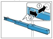
2. Place the telescopic rail on the rear pin ① and push the locking mechanism back ②.
