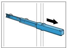
2. Move the lock in the direction of the arrow 1 and loosen the pin from the rear 2.
