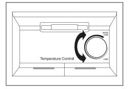
**Note:** At a room temperature above 32 °C, slightly reduce the temperature setting in the appliance.
