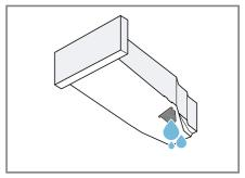
Check the condensation container filter → Page 37 regularly and clean the filter if it is dirty.
