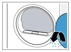
3. Remove the two-part fluff filter.
