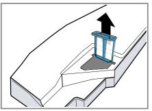
3. Clean the filter under warm, running water or in the dishwasher. 4. Slide in the filter as far as it will go.
