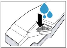
Hold the full condensation container level so that no liquid spills out.
