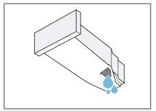
Check the condensation container filter  $\rightarrow$  Page 43 regularly and clean the filter if it is dirty. Make sure that you insert the condensation container before operating the appliance.
