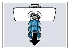
4. Press the locking catches 1 together and lift the coarse filter out ②.
