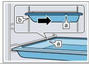
**3.** To place the accessory at the shelf positions with the pull-out rails, pull out the pull-out rails.
