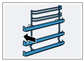
The rails fit both on the left and right sides. Shelf positions 1 and 2 are located at the bottom and shelf positions 3, 4 and 5 are located at the top. Pull out the telescopic rail towards the front.
