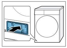
2. Close the lever for the heat exchanger.
