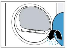
3. Remove the two-part fluff filter.
