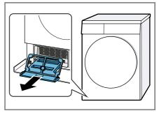
5. Clean the insert under running water and dry it off.
