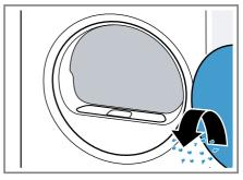
**3.** Remove the two-part fluff filter.
