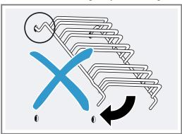
**3.** Both hooks must be inserted fully into the upper holes. Move the rail down slowly and carefully, and hook it into the lower holes.
