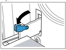
3. Close the oven door as far as the limit stop. Grip the left and right hand sides of the door with both hands. Close the door slightly more and remove it.
