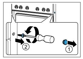
7. Remove the two screws (M4) that are uncovered when you remove the control knobs (T15).
