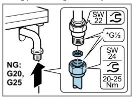
5. Open the gas connection shut-off. Carry out a leak test → Page 36.
