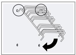
4. Hook both rails into the side walls of the oven.
