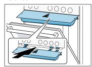
Note: There are three notches below the control panel. Insert the three lugs on the protecting plate into the three notches.
