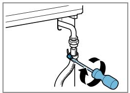
4. Open the gas connection shut-off. Carry out a leak test → Page 36.
