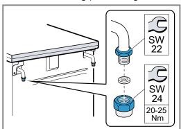
3. After changing the connection side, carry out a leak test. You can find additional information about this in the section entitled "Leak and function test" → Page 36.
