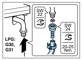
3. Fit the safety gas hose and use a pipe union or cable clamp to tighten it securely.
