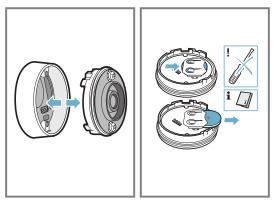
3. Insert a new battery, observing the instructions for the battery poles. Only use premium-quality CR2032 batteries.
