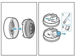
Insert a new battery, observing the instructions for the battery poles. Only use premium-quality CR2032 batteries.
