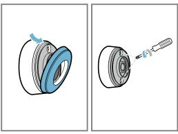
2. Open the cooking sensor lid and remove the battery from the base.
