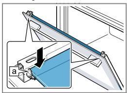
5. Open the appliance door and attach the door seal.
