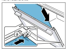
Push the intermediate pane upwards until it is in the left- and right-hand retainers a.
