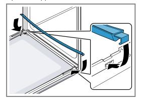
6. Slide the inner pane into the left- and right-hand retainers a.
