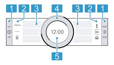
The buttons on the left- and right-hand side of the control panel have a pressure point. Pressing a button will execute its function. On appliances without a stainless steel front, the buttons are also touch-sensitive.
