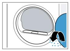
3. Remove the two-part fluff filter.
