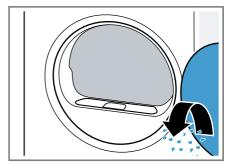
3. Remove the two-part fluff filter.
