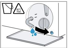
8. Firmly press on the sealing cap.
