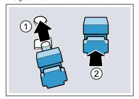
3. Hook the rear retainers with the hook into the top hole 1) and push them into the bottom hole 2.
