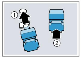
**3.** Hook the rear retainers with the hook into the top hole ① and push them into the bottom hole ②.
