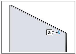
2. Insert the intermediate pane into the retainer a at the bottom 1 and push it in firmly at the top.
