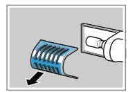
4. Replace the illuminant. Replacement illuminant: 220-240 V AC, E14 bulb holder, see the defective illuminant's wattage.
