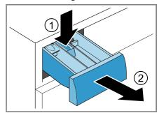
3. Pull out the insert upwards.
