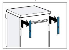
3. Undo and remove the screws in the horizontal transport strut using a T20 screwdriver
