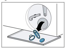
The pump cap is comprised of two parts which can be taken apart for cleaning.
