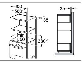
Do not fit the appliance too high up; it must be possible for accessories to be removed easily. Fit the feet.
